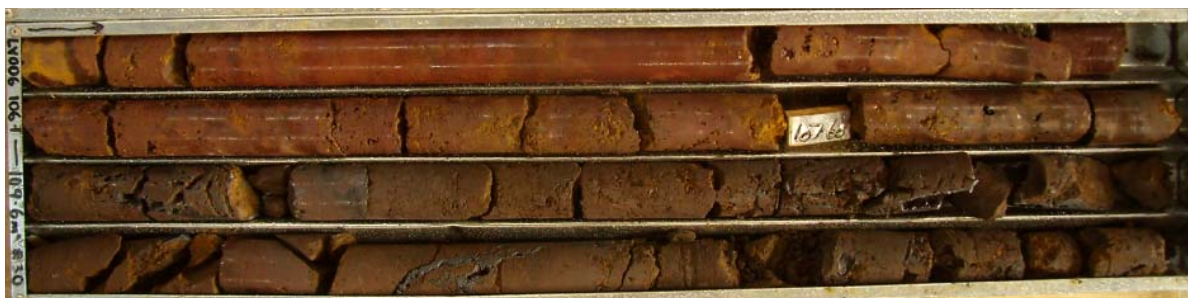
Some of the drill core from LV006 – 29.8m @ 60.1%Fe from 92.3 metres
